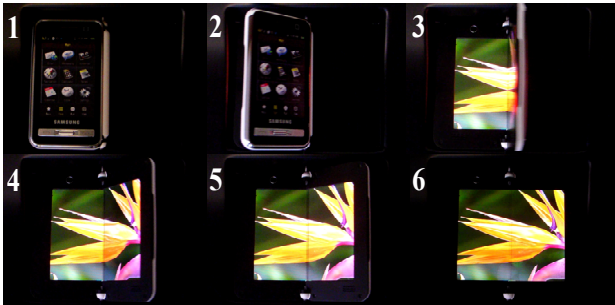
Figure 12. Successive still shots of prototype display unfolding.
